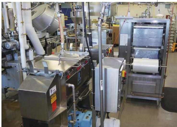
▶ **To ensure the homogeneity of various soup products in final packaging, the Heinz team pumps finished soup to a Ross ribbon blender, where continuous agitation prevents garnishes from settling. The product enters the blender through the cover and is pumped from a discharge valve beneath the blender directly to filling equipment alongside the blender.** Source: Charles Ross & Son Company.
