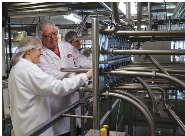
▶ **Process equipment and feed lines in the plant are interconnected through hard-piped “process zones.” Working like giant switchboards, these manifolds simplify changeover, increase production and make the plant more responsive to customer needs.** Source: Charles Ross & Son Company.
